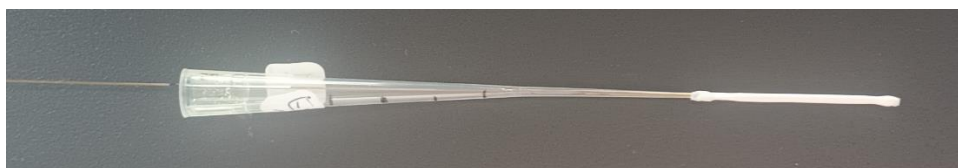
Figure 1. Microdialysis probe (length 22 mm) made of polysulfone UF membrane.
