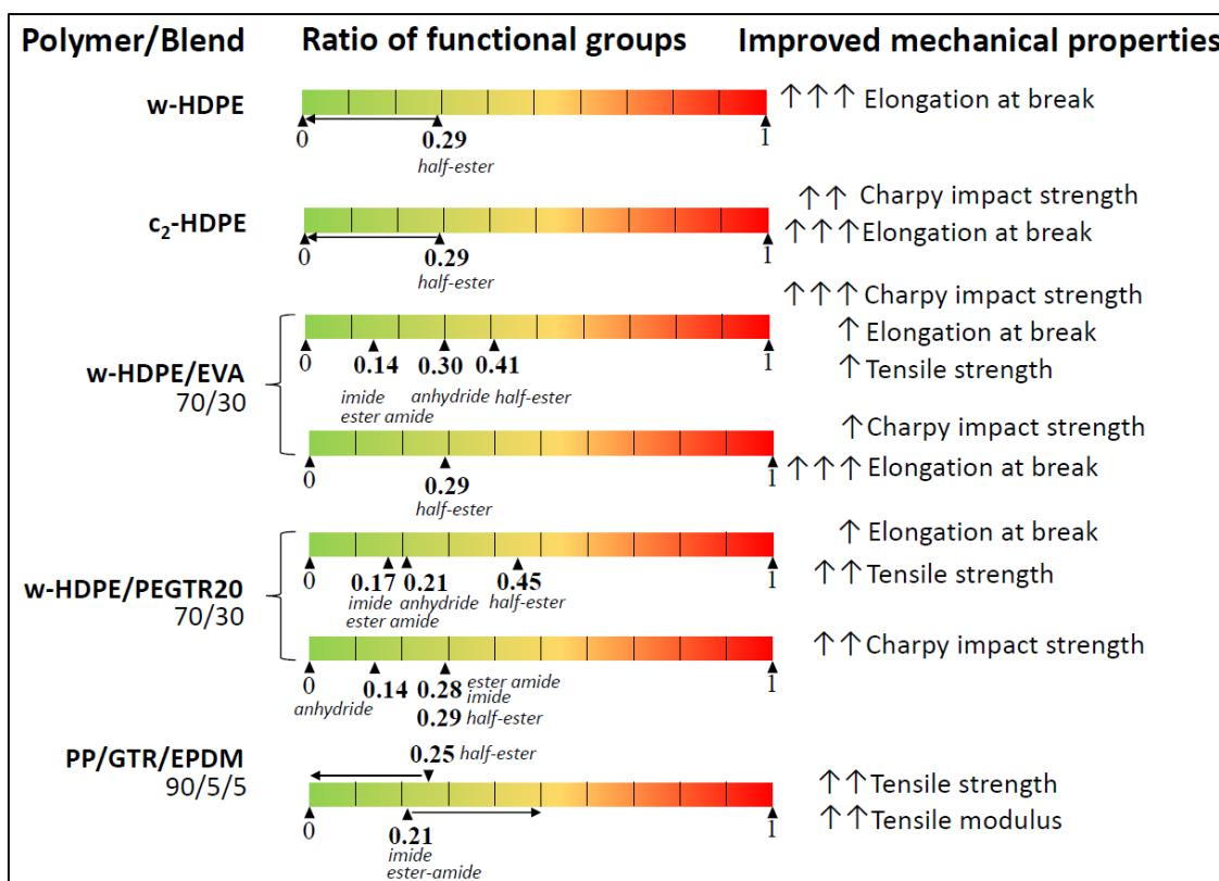
Experimental blends can be applied in any fields where there is no special requirement for purity and colour. Waste HDPE/waste elastomer based experimental blends can be used for example as a storage box, dog kennel cover, cat litter tray or a sport equipment (e.g. hockey puck), meanwhile experimental waste HDPE/EVA blends can serve as agricultural films.
