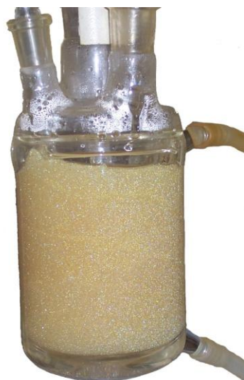
Figure 36: Mixing during neutralization
