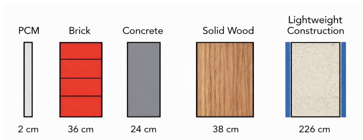
Figure 1: Comparison of the required PCM layer thickness with other structural elements of equivalent thermal storage capacity (based on Thermofoam et al. 2021.)
