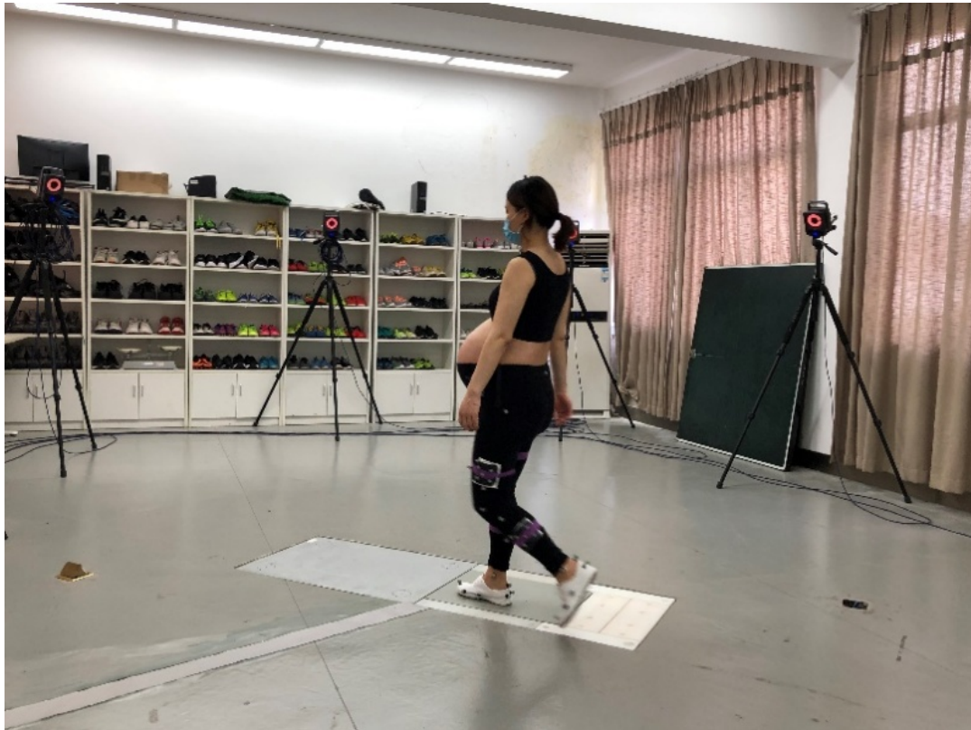
Figure 2.4. Experimental setup for gait data collection in pregnant participants using a motion capture system.
