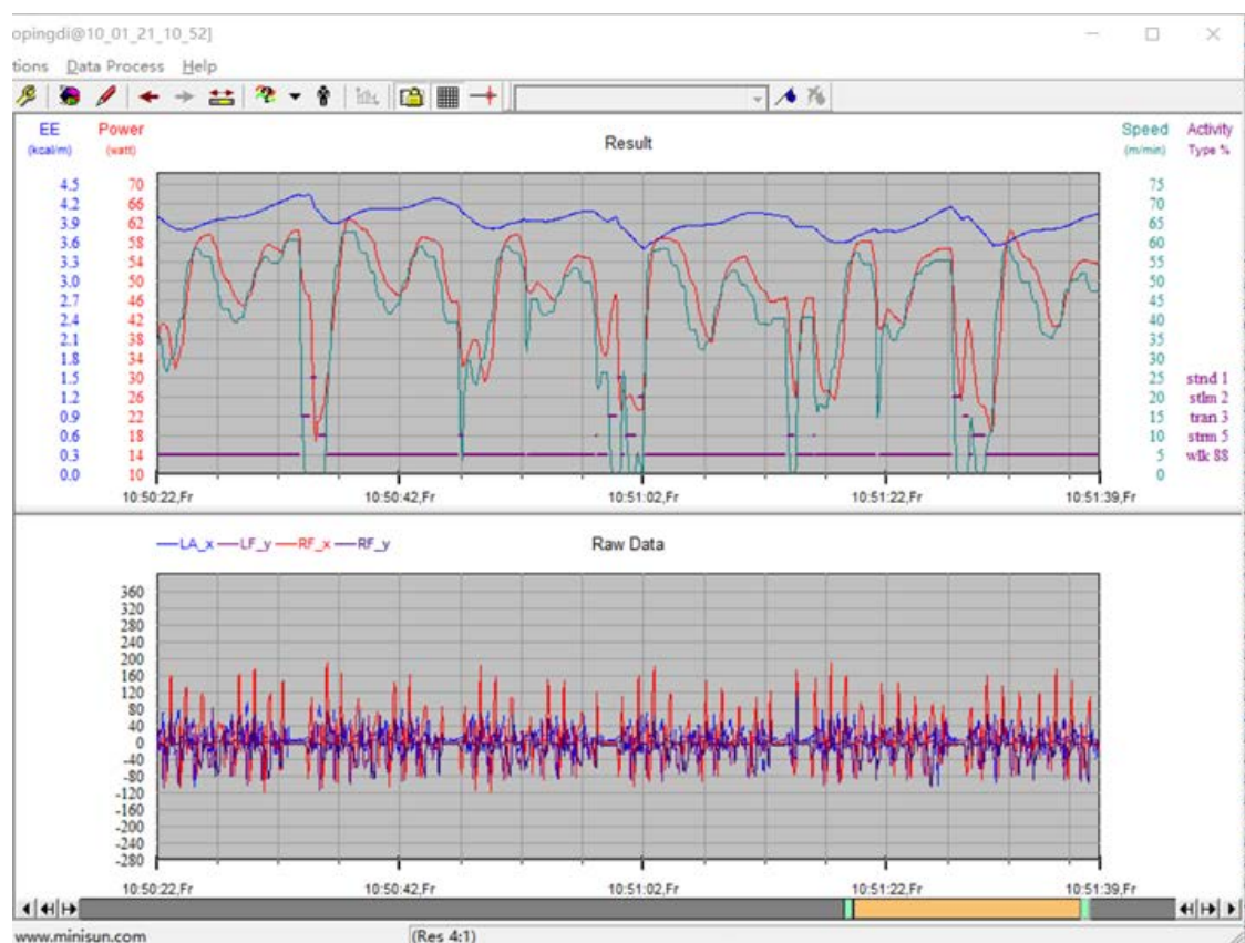
Figure 2.2. Software interface for gait-related data processing and visualization, including energy expenditure, power output, walking speed, and raw sensor signals.
