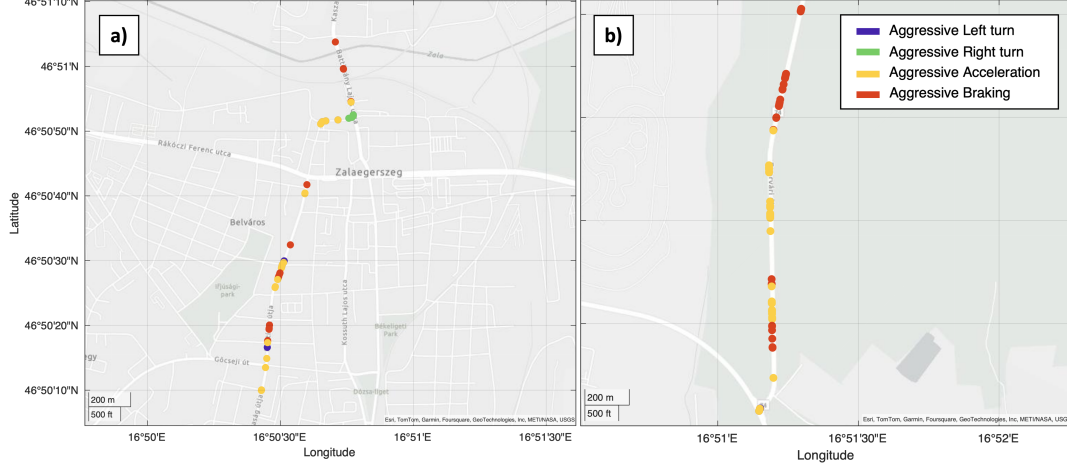
Figure 22: Measurement and classification results in urban (a) and suburban (b) environments with medium traffic intensity, for the Sedan vehicle
